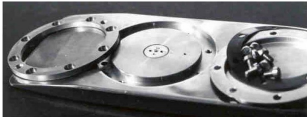
Figure 3 (left): Assembled dilatometer blade and dilatometer blade with membrane removed Figure 4 (right): Tolerances for sensing disk, feeler, and Plexiglas cylinder
