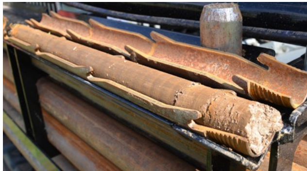
Figure 3: Finger Split Spoon Sampler [Left: opened with sample] [Right: assembled]
