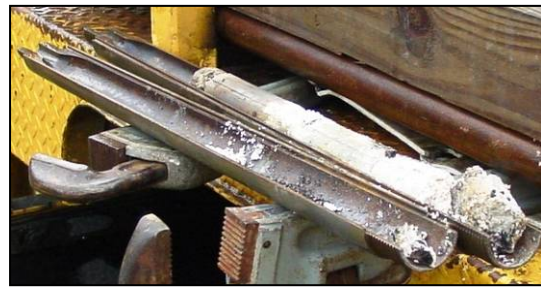
Figure 2: Split spoon SPT sampler
