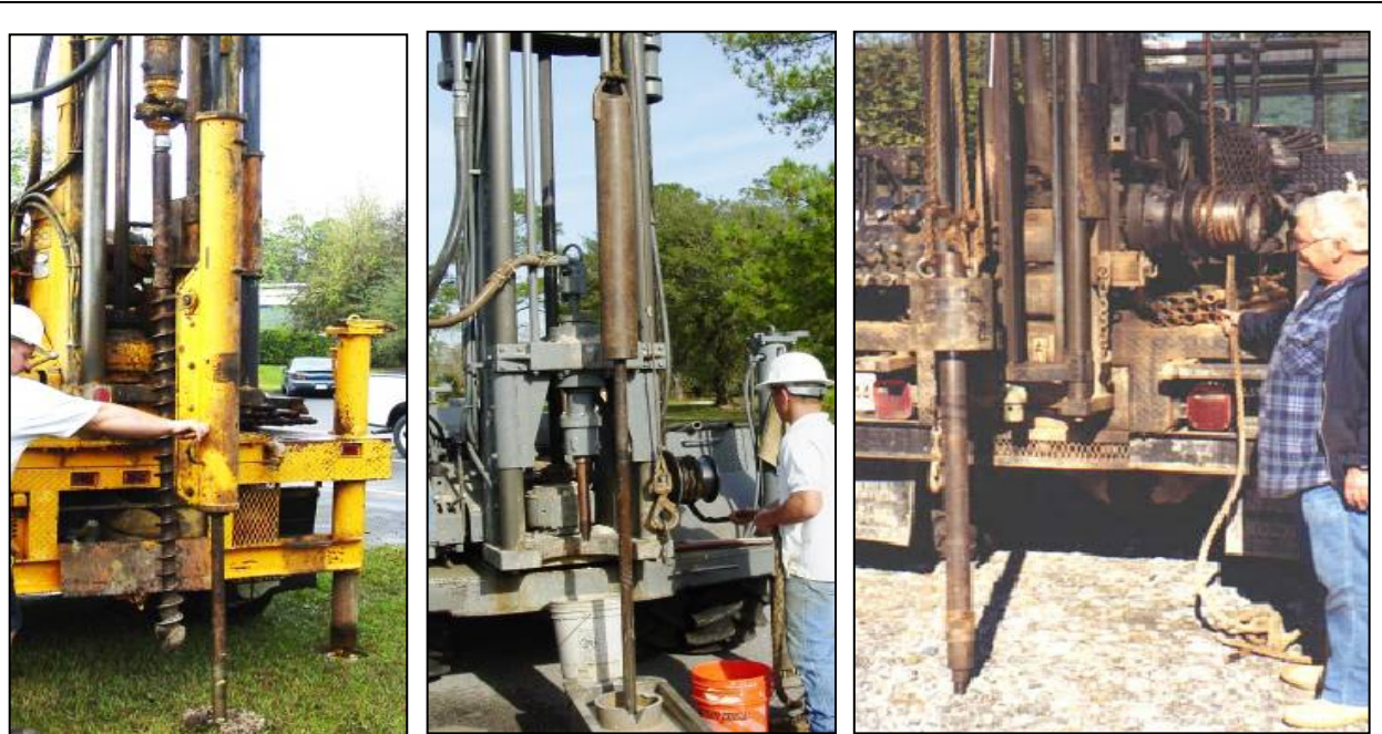
Figure 4: a) Automatic Hammer ~95% efficiency, b) Safety Hammer ~60% efficiency, c) Donut Hammer ~45% efficiency. (photo from GeoServices Corp.)
