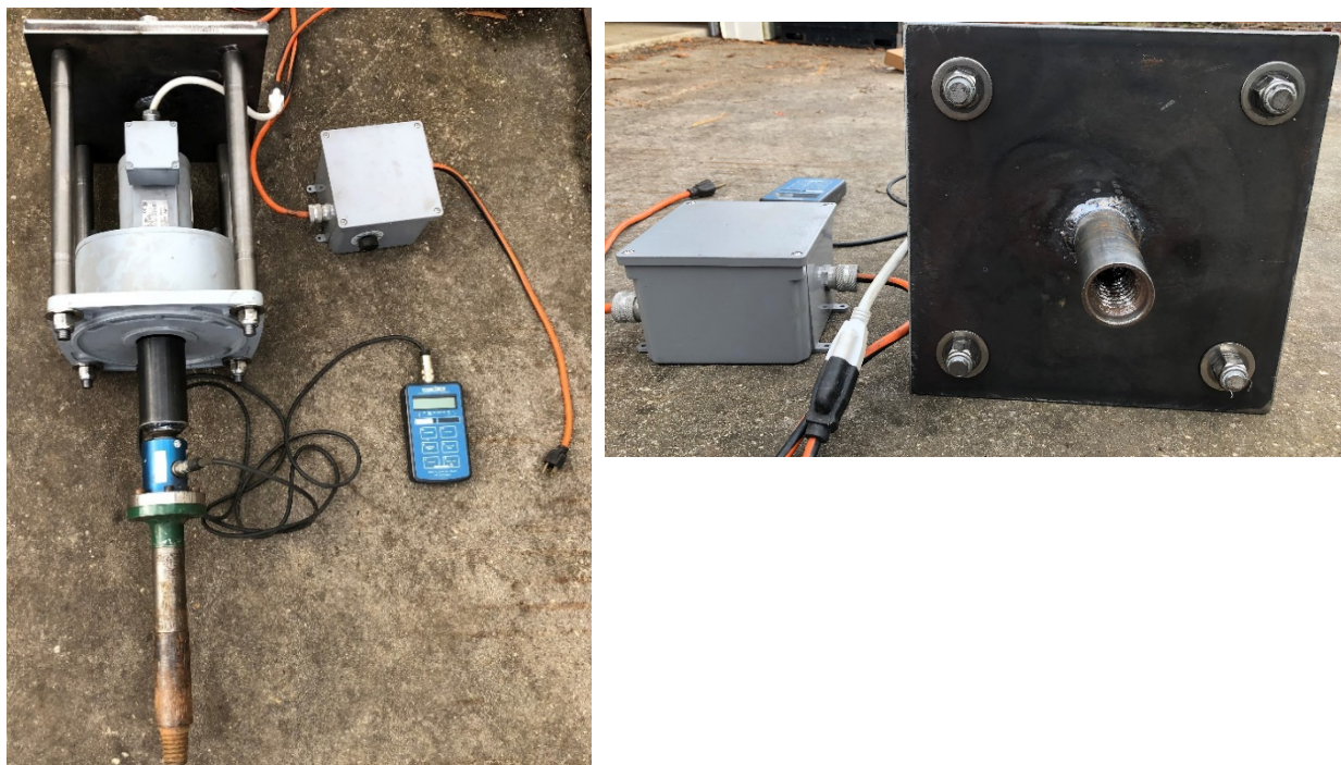
Figure 7: Electric motor SPT torque equipment (left) Top adapter for hoist cable and during test for pipe wrench to provide reaction for torque motor (right)
