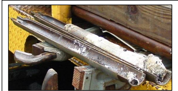
Figure 1: Split spoon SPT sampler
