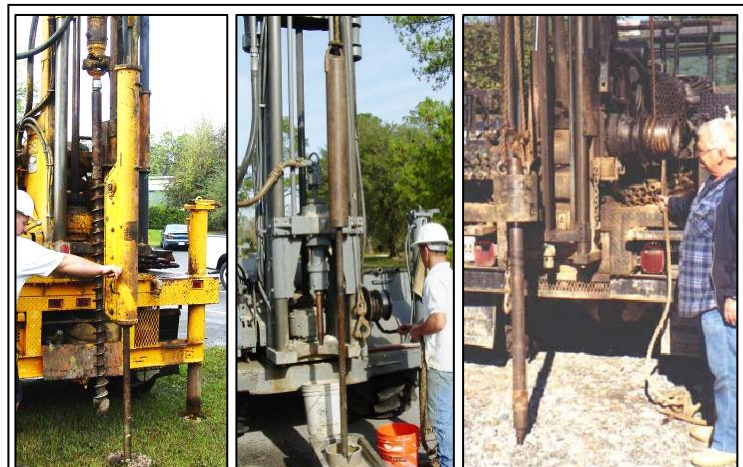
Figure 2: a) Automatic Hammer ~95% eff., b) Safety Hammer ~60% eff., c) Donut Hammer ~35% eff. (photo from GeoServices Corp.)
