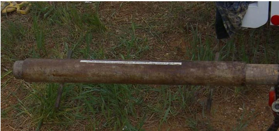
Figure 7: Pressuremeter probe inside thick-walled steel calibration tube
