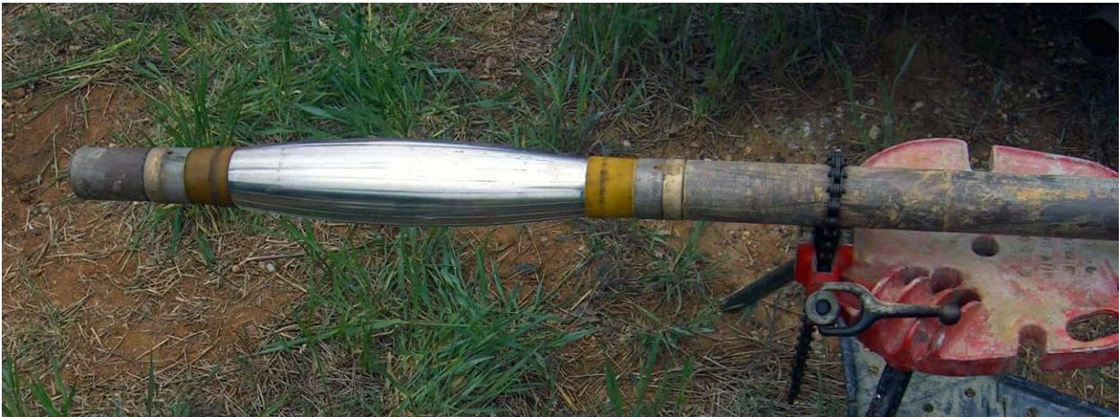
Figure 8: Membrane calibration at fully expanded volume of  $1600 \text{ cm}^3$
