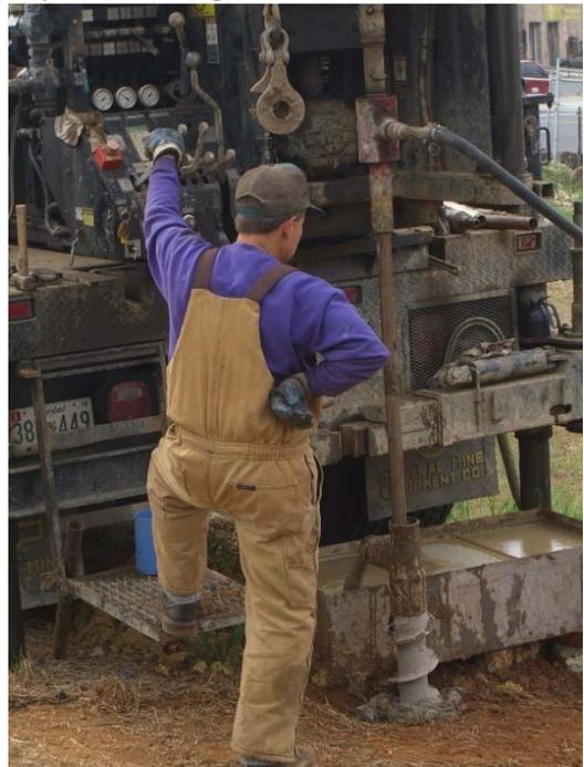
Figure 5: Ronald Stidham drilling a pressuremeter test hole
