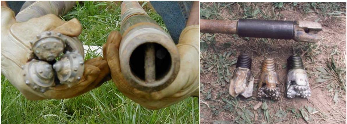
Figure 4a-b: Drill bits used to make the pressuremeter test hole
