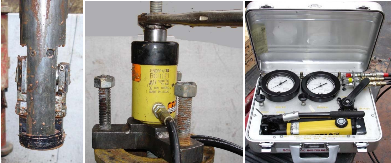
Figure 3: Rock borehole shear test equipment
