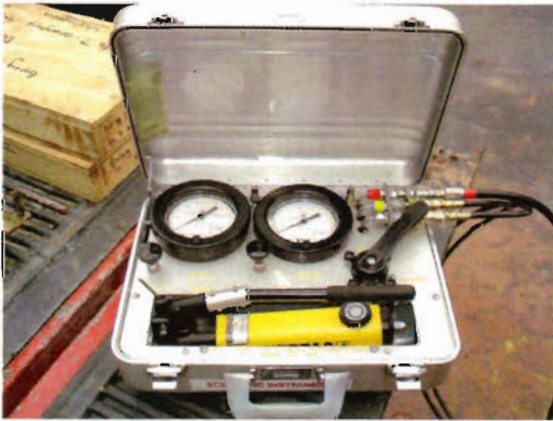
Figure 2. Rock borehole shear control unit.
