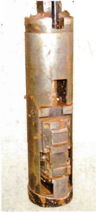
Figure 1. Rock borehole shear head.
