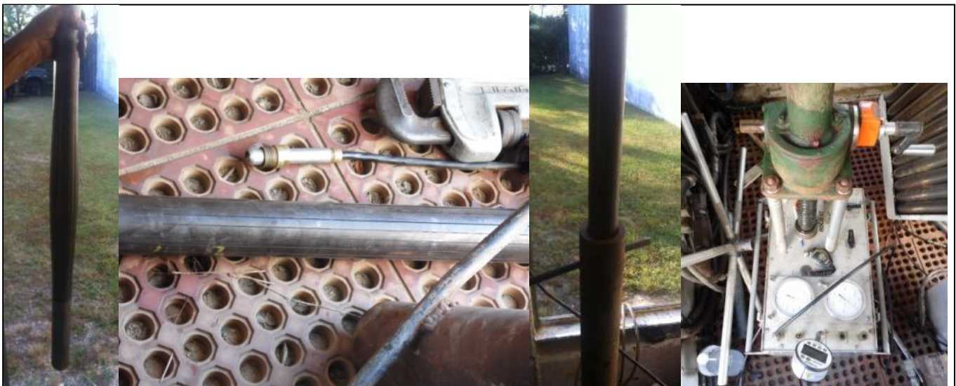
Figure 1: Photo of a) expanded pushed-in PMT b) close-up of longitudinal 0.254 mm wide slots c) lowering slotted PMT into thick walled steel calibration pipe d) Texam pressuremeter control unit
