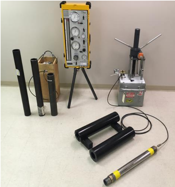
Figure 1. Equipment used: TC and MC PMT, N-size probe, steel calibration tube, and polymer TSTs
