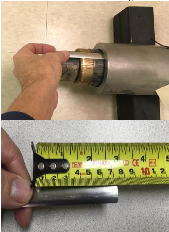
Figure 5. Measuring CL with a steel strip
