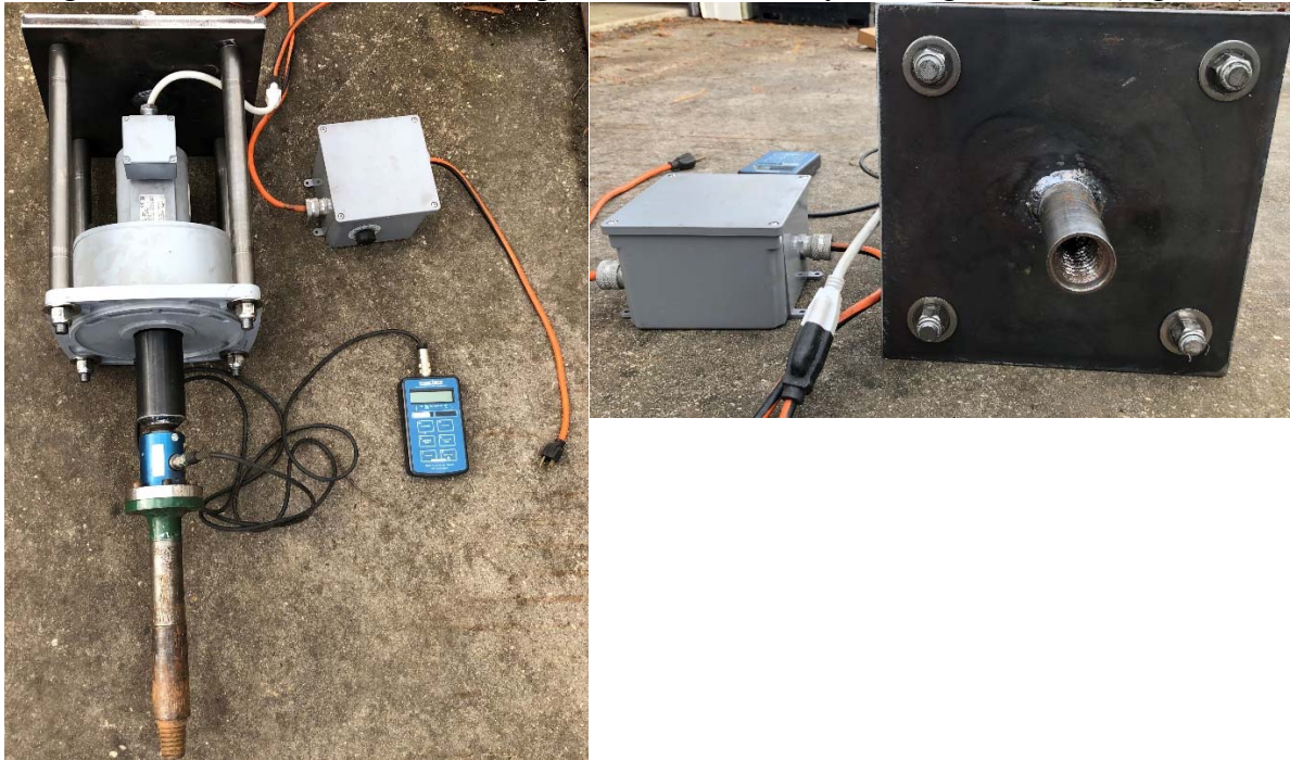
Figure 6: Electric motor SPT torque equipment (left) Top adapter for hoist cable and during test for pipe wrench to provide reaction for torque motor (right)
