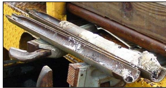
Figure 2: Split spoon SPT sampler
