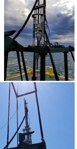
hydraulic piston raises the hammer until it trip-releases sending the high energy seismic wave into the soil. Our "box lid" seismic plate embeds into the river mudline soils and creates excellent coupling to transfer the shear waves through the soil to our seismic DMT geophones. To generate additional energy, the hydraulic piston can also pull against elastic bands.
