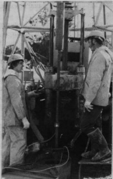
(b) The SPT hammer-rod system with load cell in place
