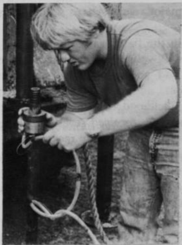
(a) Screwing the dynamic load cell into the string of rods
