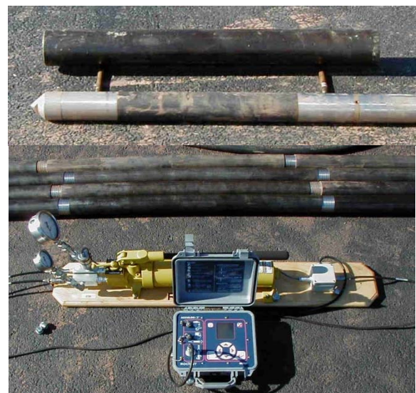
Figures 2 and 3: Rock pressuremeter probe/calibration tube and hydraulic piston/data logger
