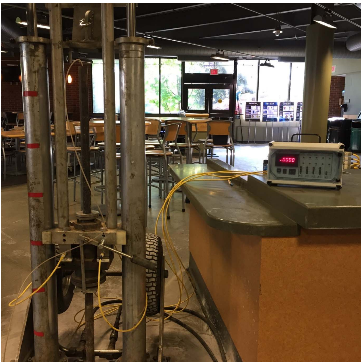
Portable push rig for dilatometer testing at Phillips Hall at James Madison University in Harrisonburg, Virginia
