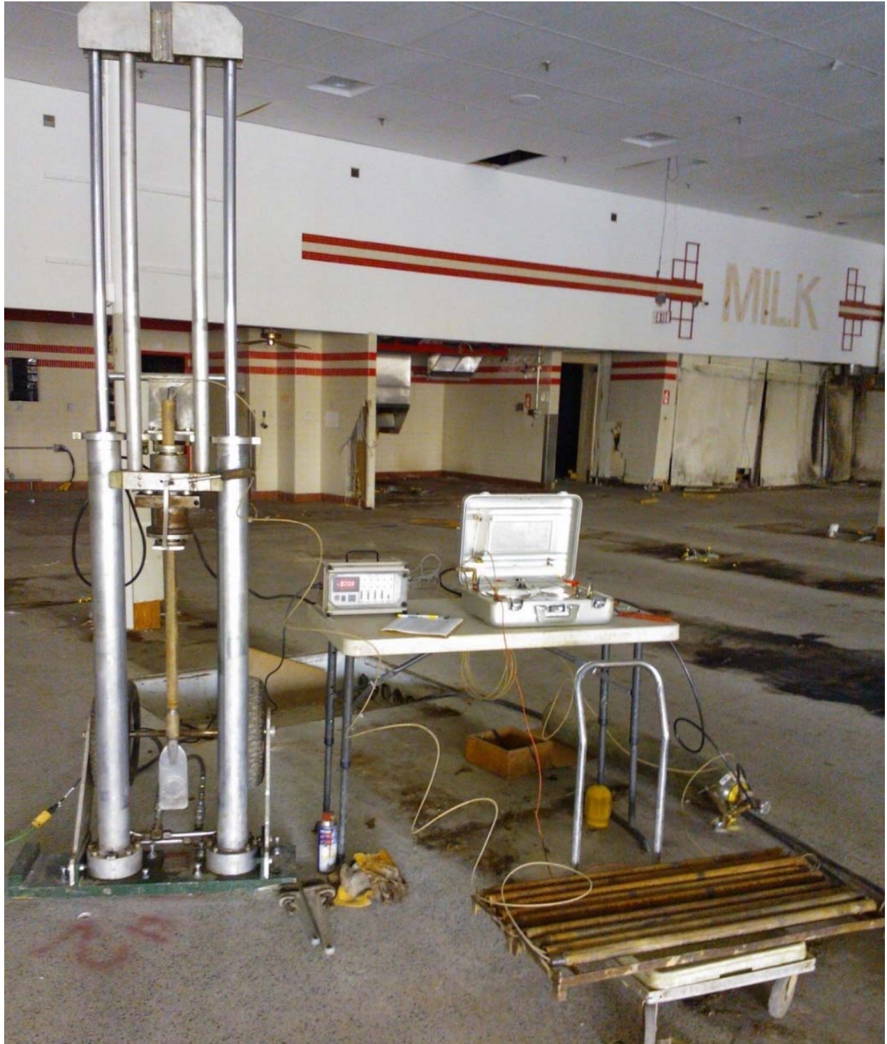
Portable push rig set-up for dilatometer testing inside an existing warehouse
