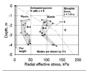
Typical data spreads in uniform soil, at a boundary between plastic remolded and elastic stress near a Rammed Aggregate Pier <sup>TM</sup>.
