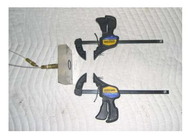
**38. Removing pressure lines and cleaning the Blade.** The standard pressure line length is 75 ft ((22 m). After testing is completed, soil can be flushed from the inner parts of the Blade head by removing the aluminum top cylinder and steel cap as shown in the photo, and sliding them up the line. The connector and lines then may be flushed and cleaned. The hollow U-shaped reinforcing rib optionally may be removed from the back of the Blade for cleaning.
