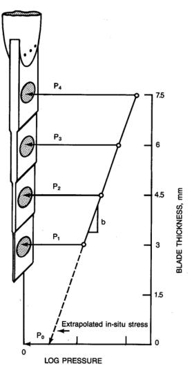
15. The pressure cells are pneumatic to avoid electrical problems in a wet, pressured environment below a groundwater table. The patented cells operate as follows:
