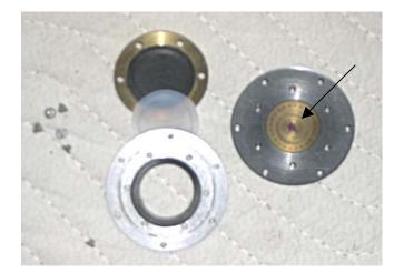
Inside a pressure cell. Arrow shows the ridge separating two chambers in the cell.
