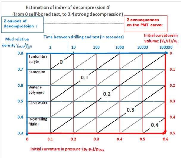
Figure 1. Estimation of the degree of decompression  $d$ , from 0 for a fully undecompressed test (self-boring pressuremeter) to 0.4 for a test in highly decompressed or remoulded soil.
