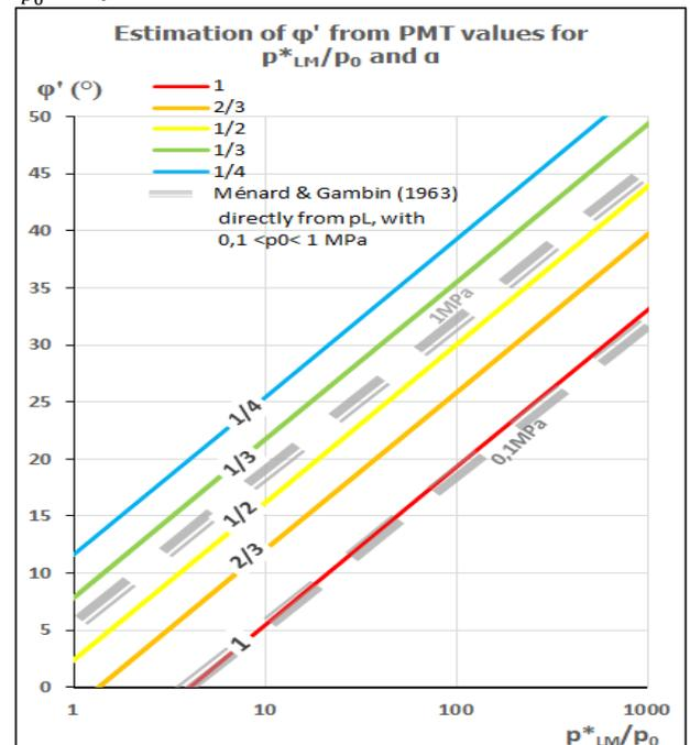
Figure 4. Estimation of  $\phi'$  from Pressuremeter test.
