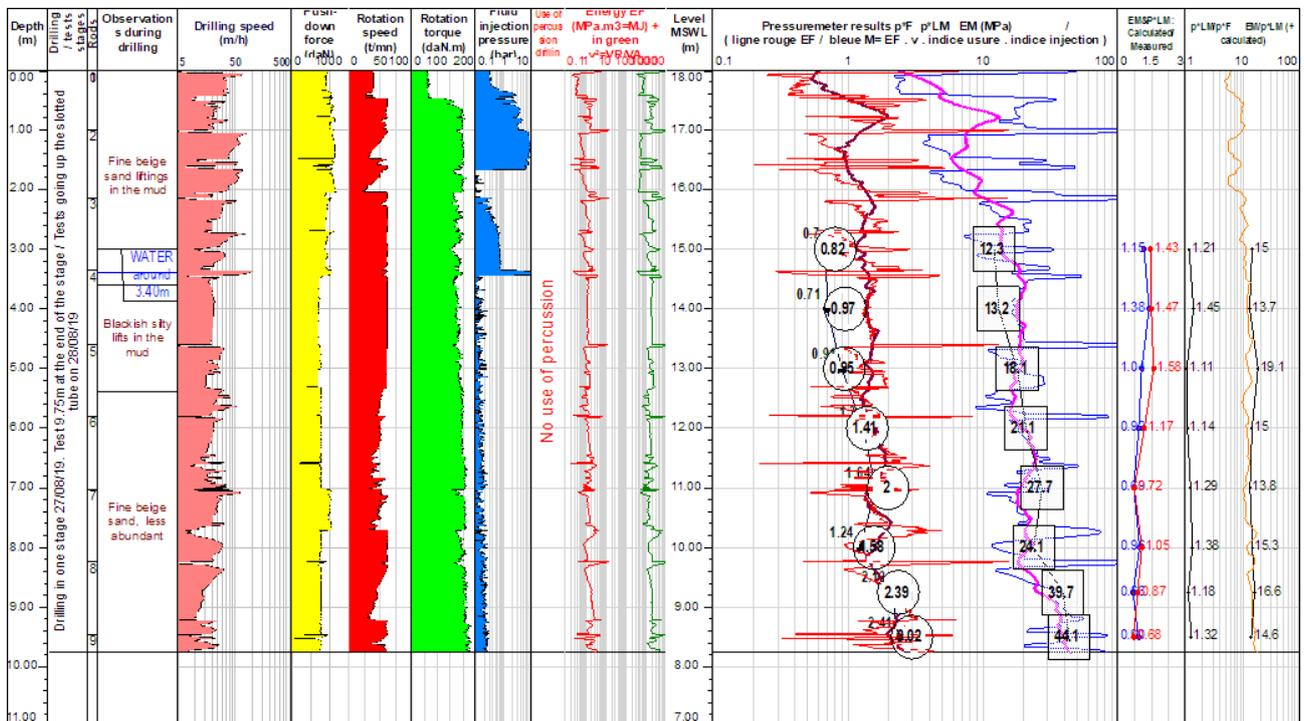
**Figure 6.** An example of interpretation of drilling parameters during self-boring of slotted casing together with the PMT tests made inside (Staf method).
