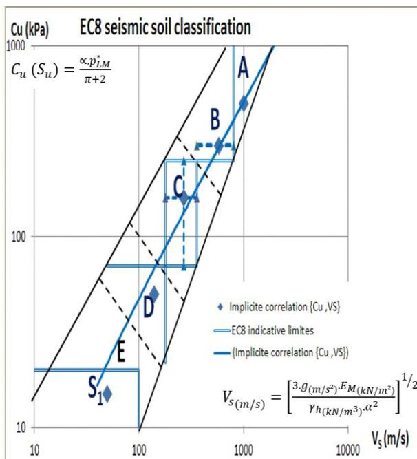
Figure 3. Use of Pressuremeter correlations for EC8 seismic soil classification [ $V_s$  |  $S_u$ ].
