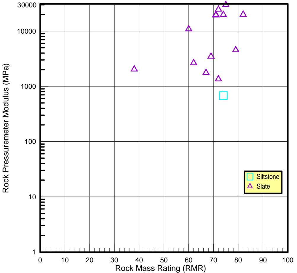
Figure 3. Pressuremeter rock modulus versus RMR comparison
