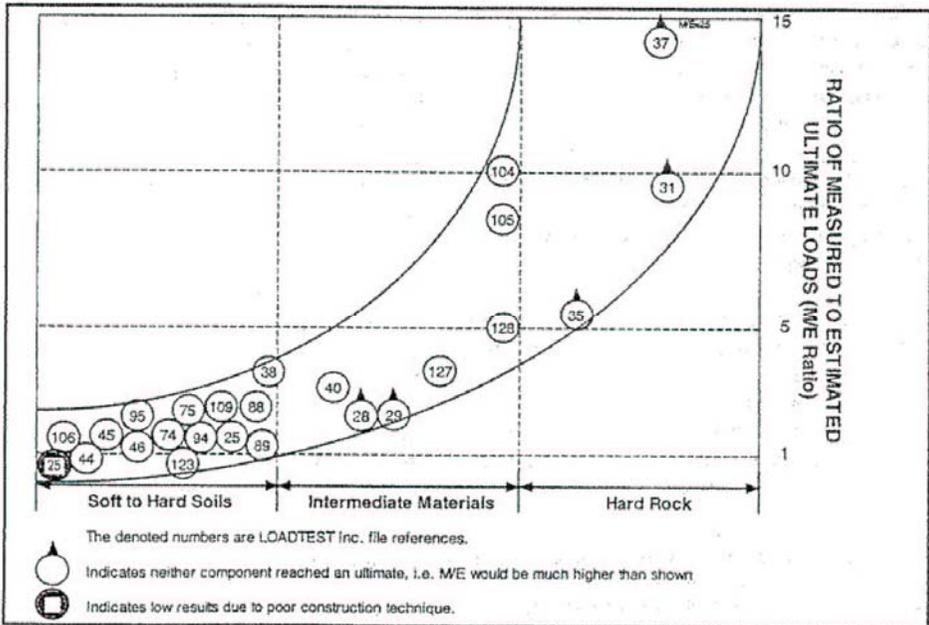
Figure 1. Underestimating rock capacity (Schmertmann and Hayes, 1997)
