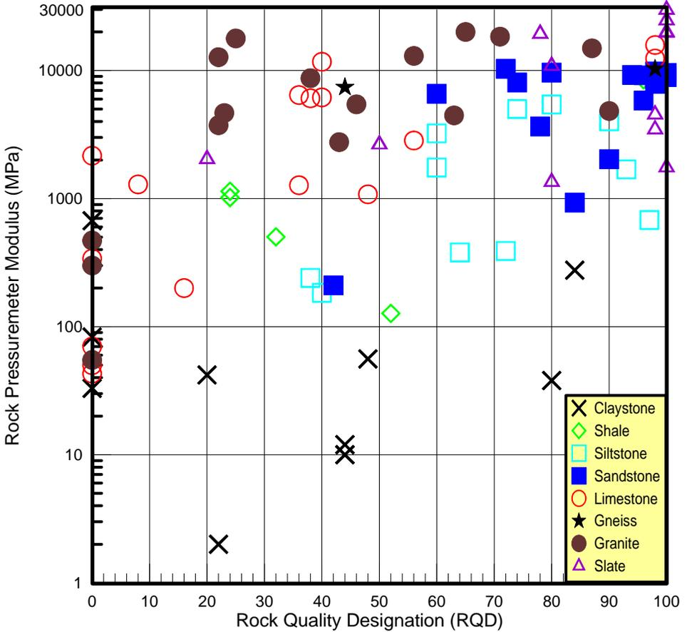
Figure 2. Pressuremeter rock modulus versus RQD comparison
