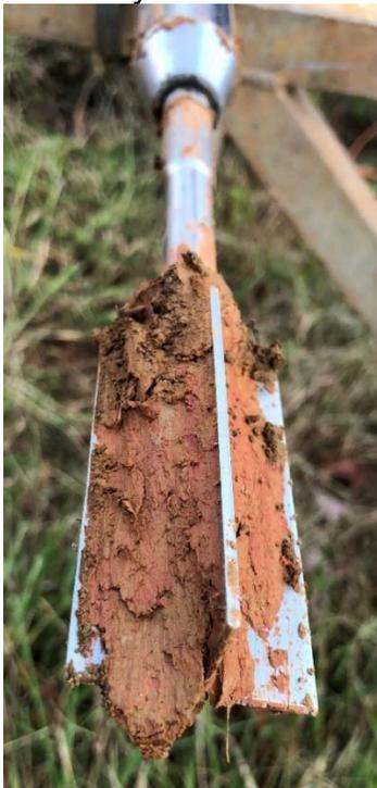
Figure 3: Small vane with stiff clay adhering to it after removal
