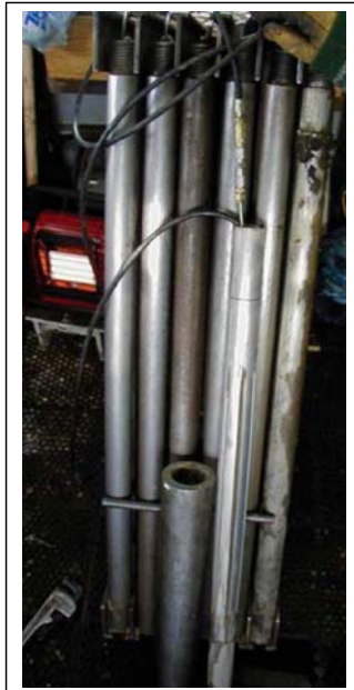
Figure 2: Push-in pressuremeter showing tubing quick-connect and calibration tube
