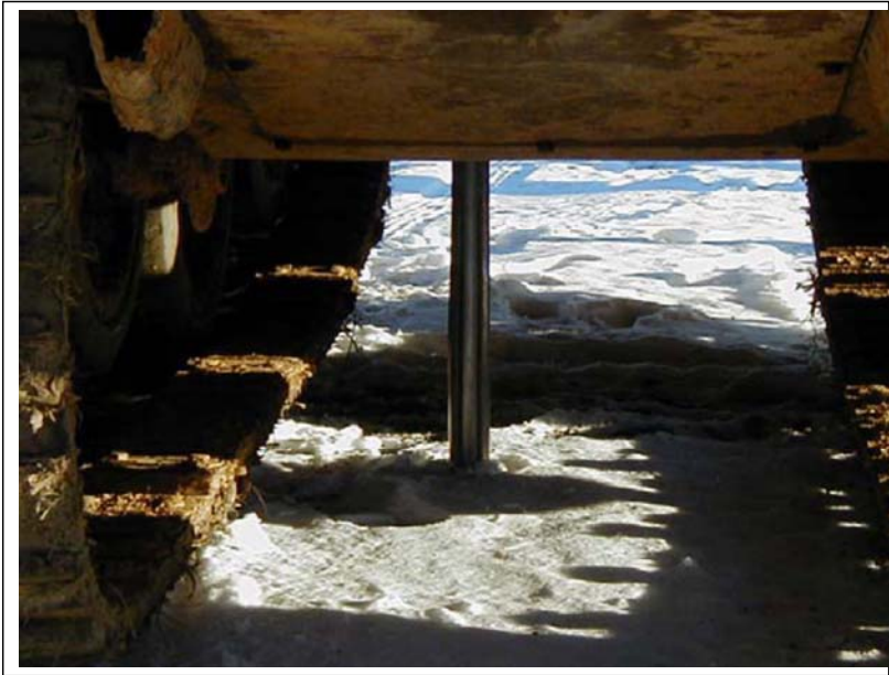
Figure 1: Push-in pressuremeter being pushed into soil
