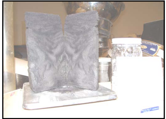
Figure 1: “Undisturbed” Fly Ash Sample: Evidence of Vertical Mixing
