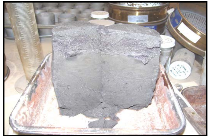
Figure 2: “Undisturbed” Fly Ash Sample: Evidence of Compression During Sampling
