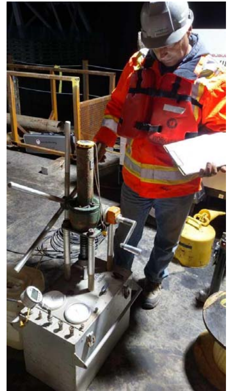
Figure 2: Performing a pressuremeter test
