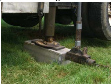
Figure 7: Seismic Pendulum Hammer Striking Aluminum Block with Rubber Pad Focusing Energy into the Ground
