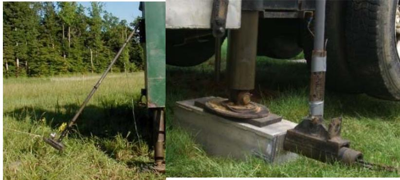
Figure 6: Horizontal strike to create seismic shear wave
