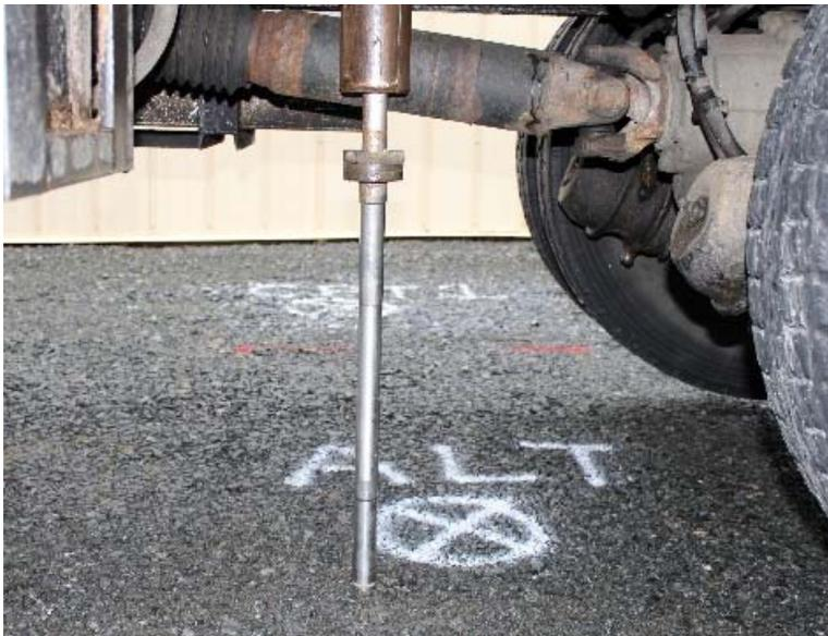
Figure 4 shows the start of a CPTU sounding with a 10 cm<sup>2</sup> piezocone, friction reducer, rubber rod wiper to keep soil below and out of the truck work space, and lateral supporting guide tube to prevent rod buckling.
