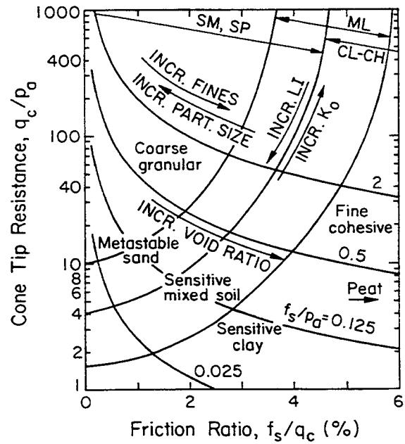
Figure 2-6. Soil Classification by Fugro Electric Friction CPT
