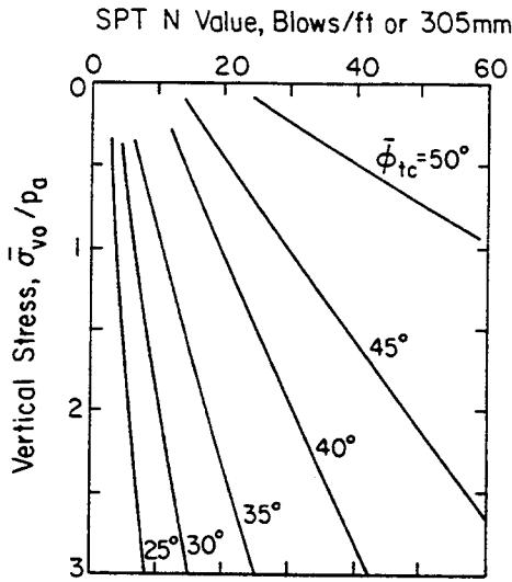
Figure 4-13. N versus  $\bar{\phi}_{tc}$  and Overburden Stress
