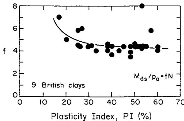
Figure 6-9. SPT Constrained Modulus Coefficient  $f$  versus PI
