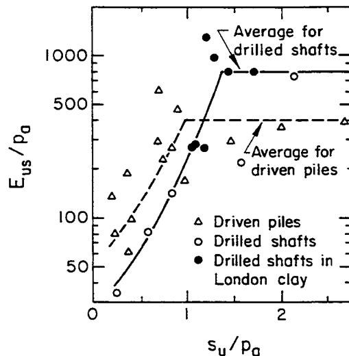
Figure 5-9. Undrained Modulus for Deep Foundations in Compression
