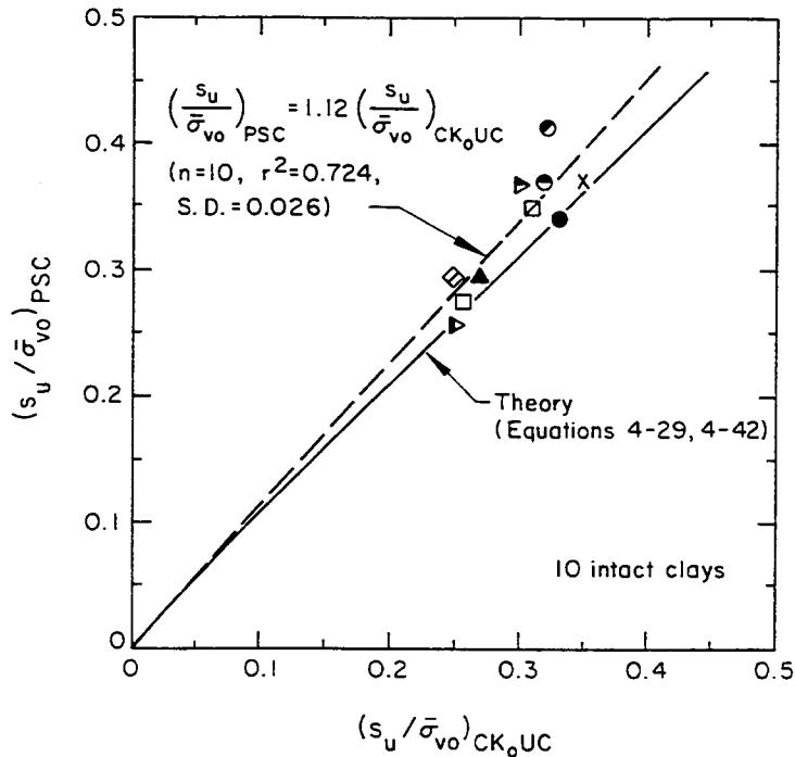
Figure 4-38. Comparison of Undrained Strength Ratios from PSC and  $CK_oUC$  Tests
