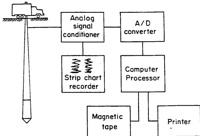
Figure B-3. Electric CPT Data Acquisition System
