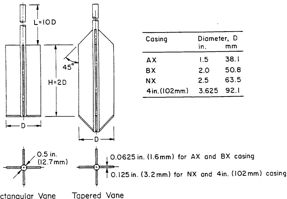
Figure E-1. Vane Geometries and Sizes
