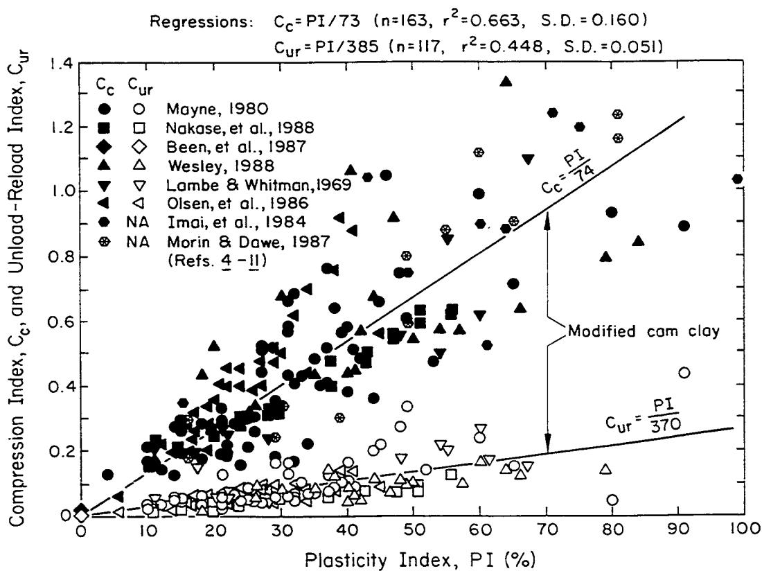
Figure 6-4. Compression and Unload-R reload Indices versus PI
