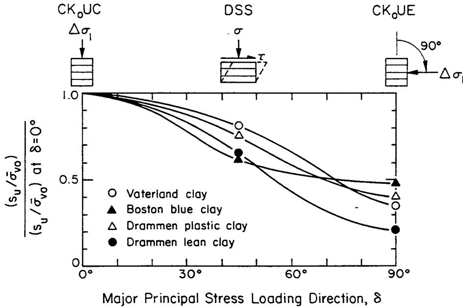
Figure 4-40. Effect of Loading Direction on  $s_u$
