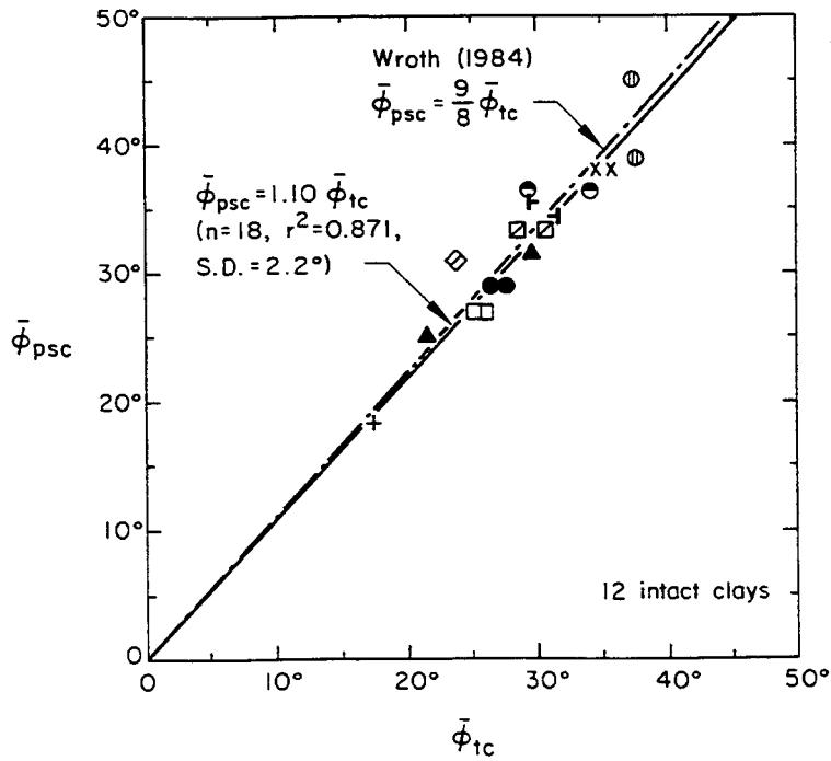
Figure 4-22.  $\bar{\phi}_{psc}$  versus  $\bar{\phi}_{tc}$  for NC Clays
