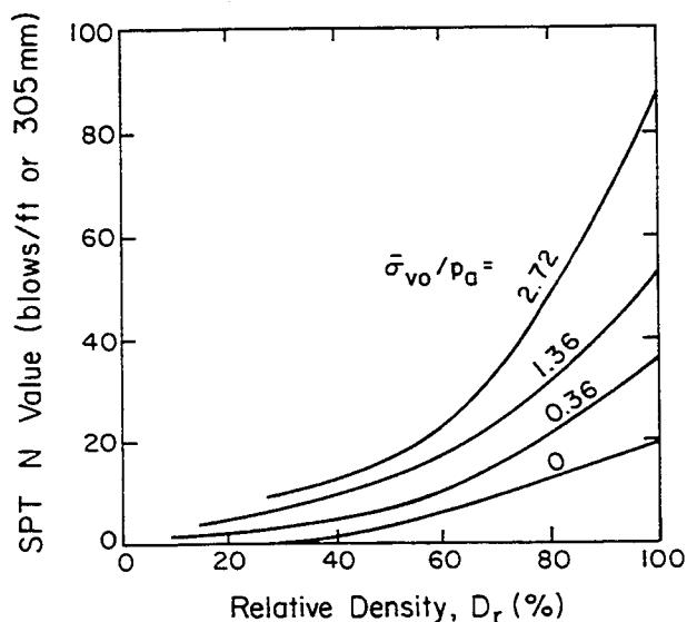
Figure 2-13. Effect of Overburden Stress and D<sub>r</sub> on SPT N Value
