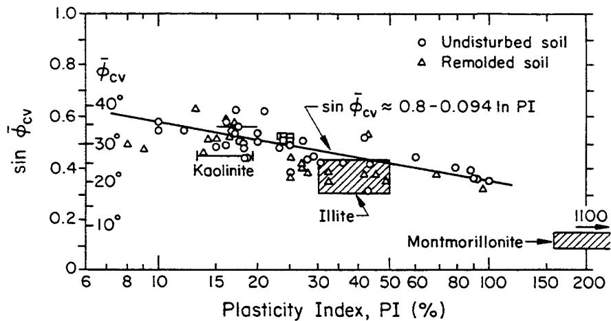
Figure 4-20.  $\bar{\phi}_{cv}$  for NC Clays versus PI
