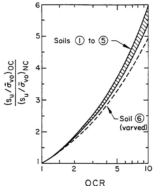
Figure 4-34. Normalized  $s_u/\bar{\sigma}_{vo}$  versus OCR
