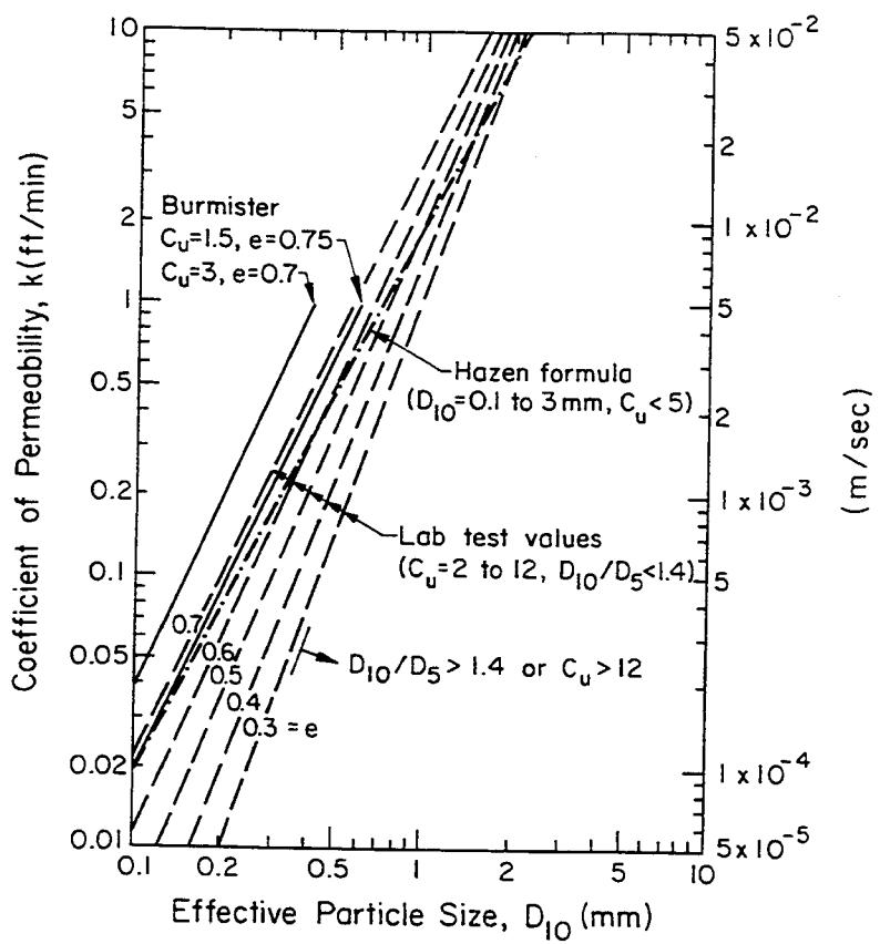
Figure 7-1. Coefficient of Permeability versus Particle Size
