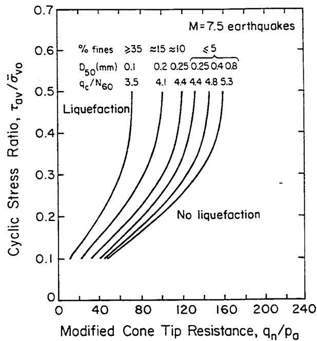
Figure 8-2. Liquefaction Resistance Correlated Indirectly with CPT Results
