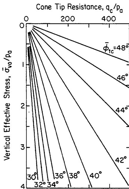
Figure 4-14.  $q_c$  versus  $\bar{\phi}_{tc}$  and Vertical Stress for NC, Uncemented, Quartz Sands
