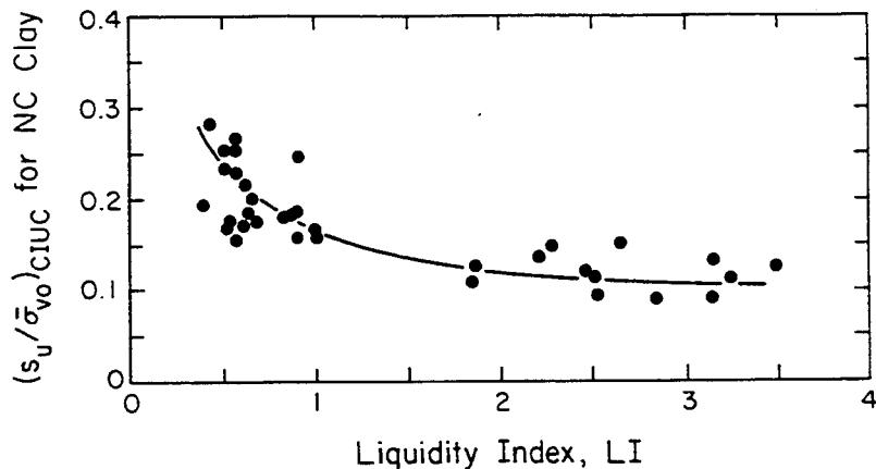
Figure 4-27.  $s_u/\bar{\sigma}_{vo}$  for NC Clay versus Liquidity Index
