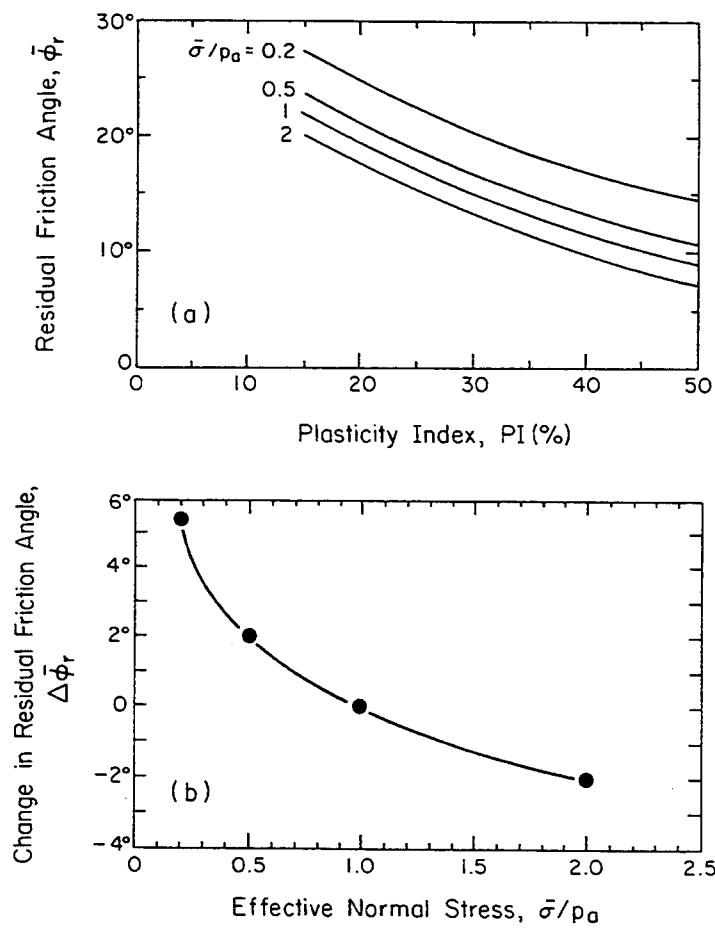
Figure 4-25.  $\bar{\phi}_r$  for Amuay Soils
