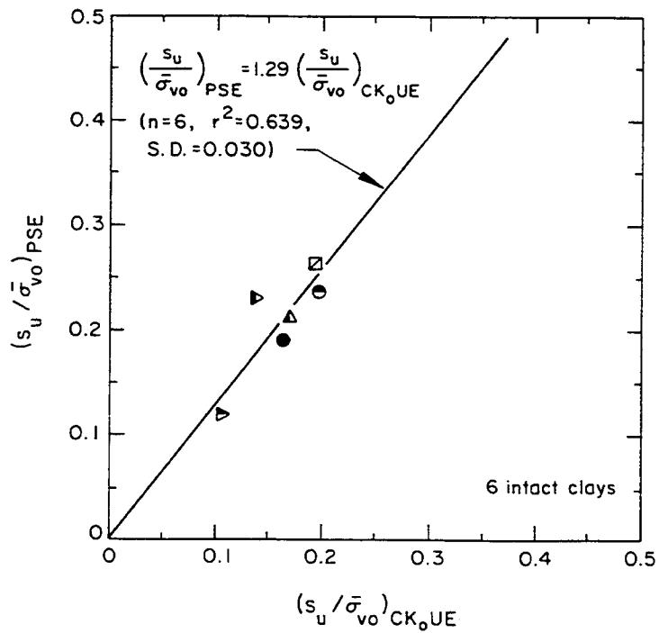
Figure 4-39. Comparison of Undrained Strength Ratios from PSE and  $CK_oUE$  Tests
