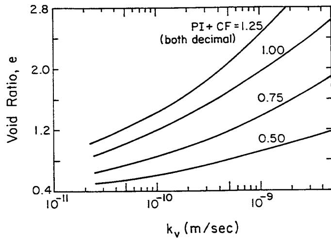
Figure 7-3. Vertical Coefficient of Permeability for Clay
