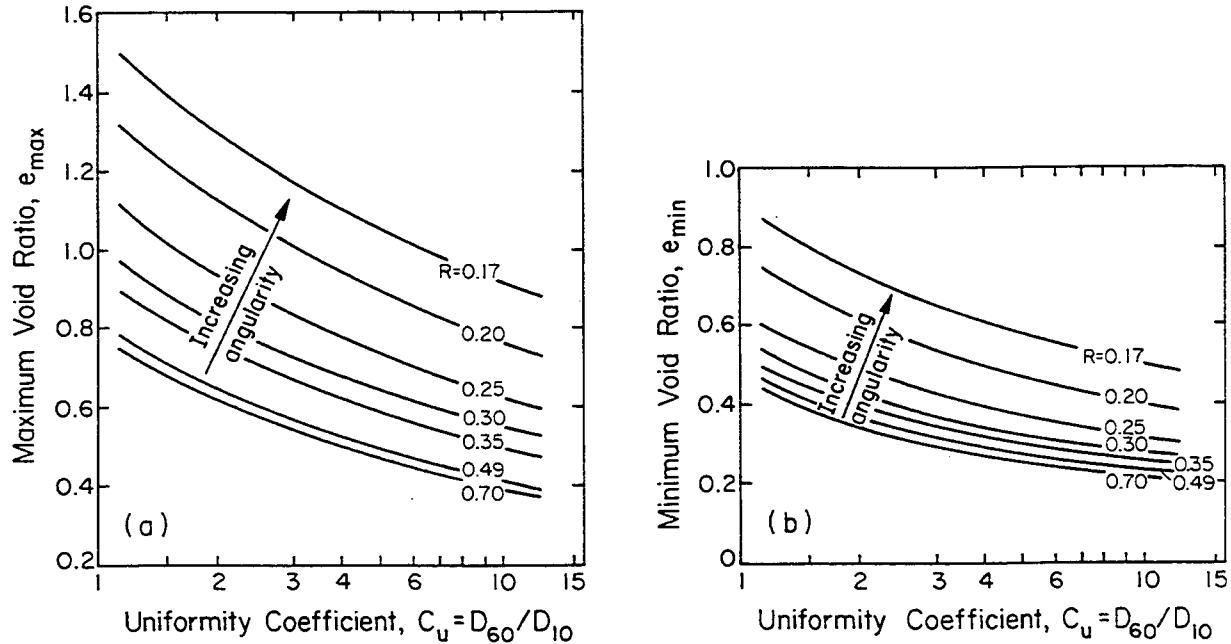
Figure 2-3. Generalized Curves for Estimating  $e_{\max}$  and  $e_{\min}$
