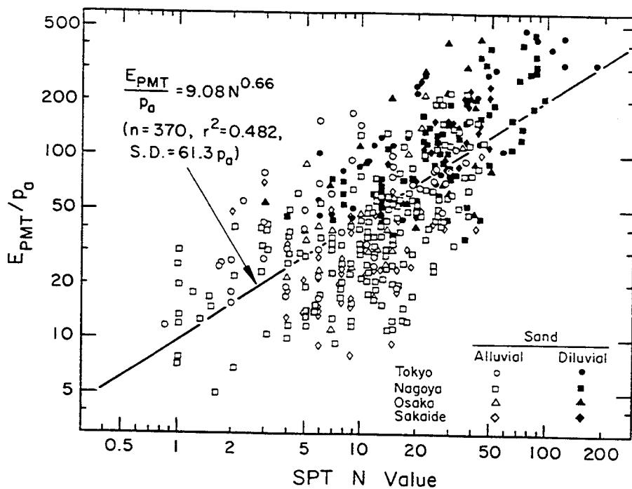
Figure 5-14. PMT Modulus of Sand versus N Value
