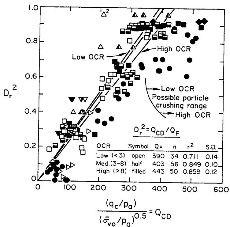
Figure 2-26. Calibration Chamber Data on OC Sands
