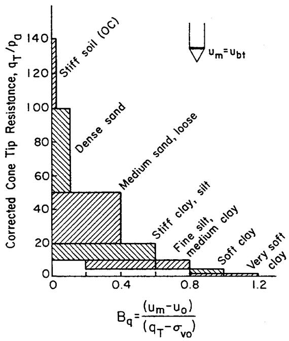
Figure 2-9. Soil Classification Based on  $q_T$  and  $B_q$
