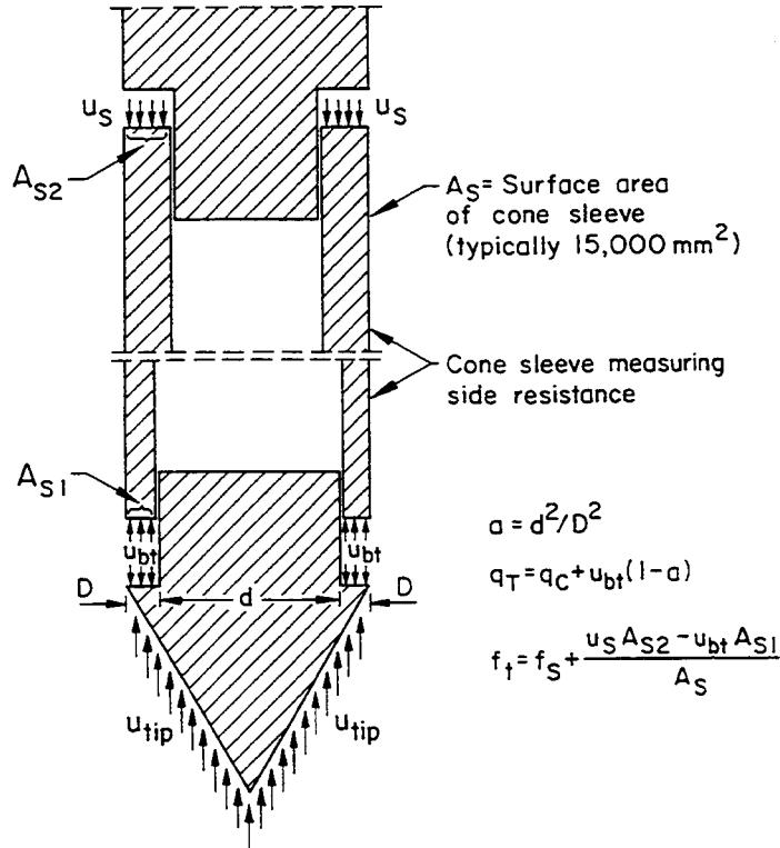
Figure 2-11. Unequal End Areas of Electric Friction Cone
