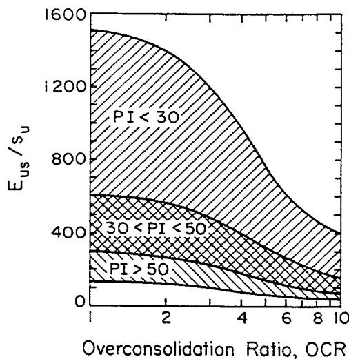
Figure 5-6. Generalized Undrained Modulus versus OCR and PI
