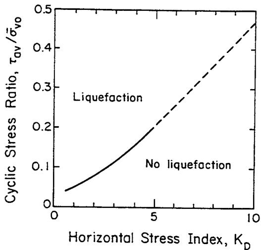
Figure 8-4. Liquefaction Resistance Correlated with DMT  $K_D$
