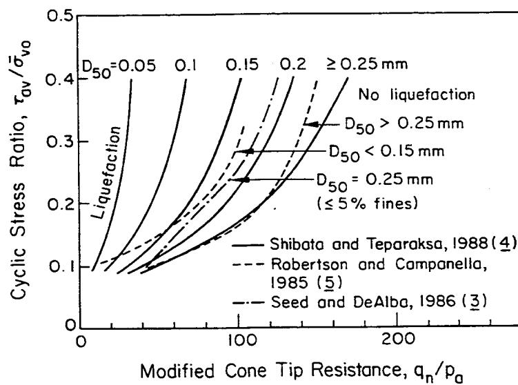
Figure 8-3. Liquefaction Resistance Correlated Directly with CPT Results
