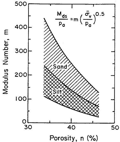
Figure 6-14. Modulus Number for NC Silts and Sands
