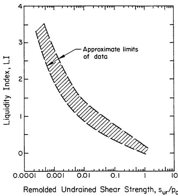
Figure 4-29. Remolded Undrained Shear Strength versus LI
