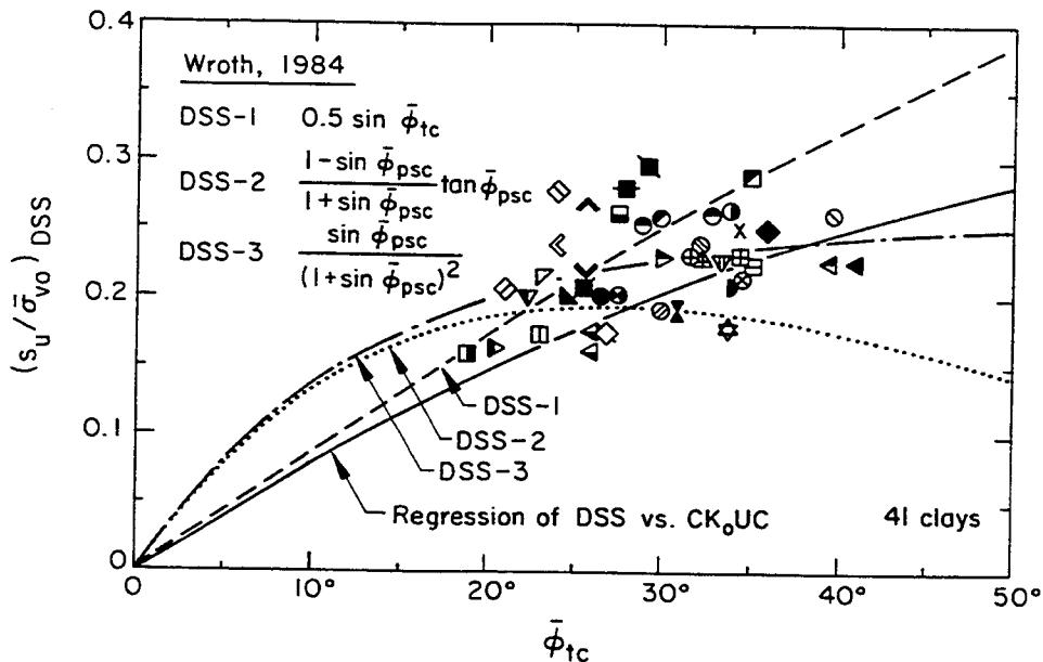
Figure 4-41. Undrained Strength Ratio from DSS versus  $\bar{\phi}_{tc}$
