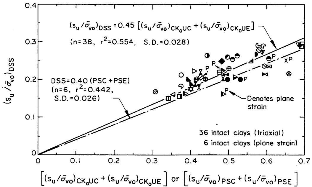
Figure 4-43. Comparison of Undrained Strength Ratios from DSS,  $CK_o UC$  and  $CK_o UE$ , and PSC and PSE Tests
