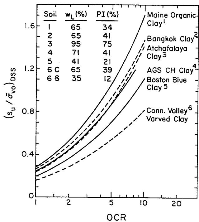
Figure 4-33.  $s_u/\bar{\sigma}_{vo}$  versus OCR
