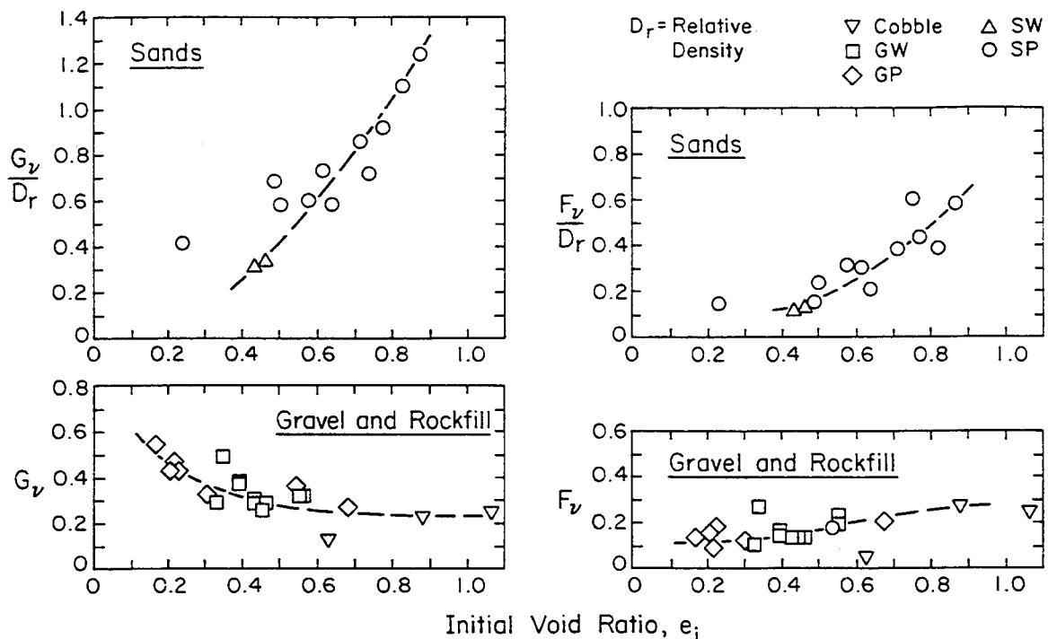
Figure 5-2. Drained Poisson's Ratio Parameters for Granular Soils
