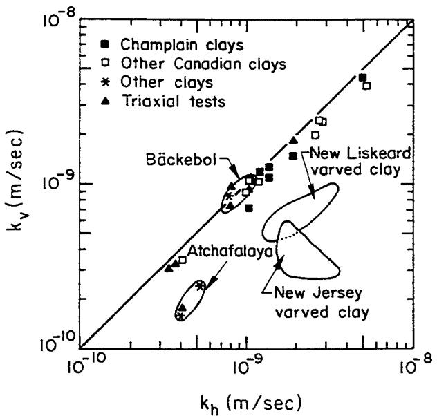
Figure 7-4. Permeability Anisotropy for Various Natural Clays
