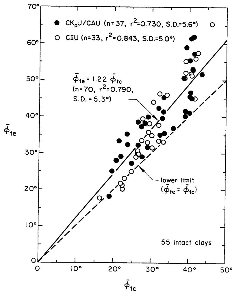
Figure 4-23.  $\bar{\phi}_{te}$  versus  $\bar{\phi}_{tc}$  for NC Clays
