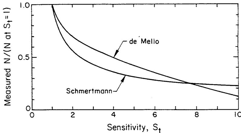
Figure 4-51. Apparent Decrease of N with Increasing Sensitivity
