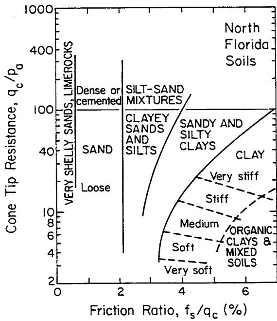
Figure 2-5. Soil Classification by Mechanical Friction CPT
