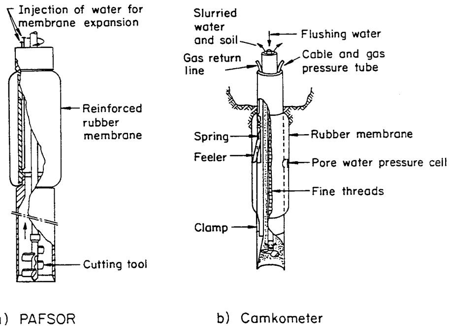
Figure C-3. Self-Boring Pressuremeters
