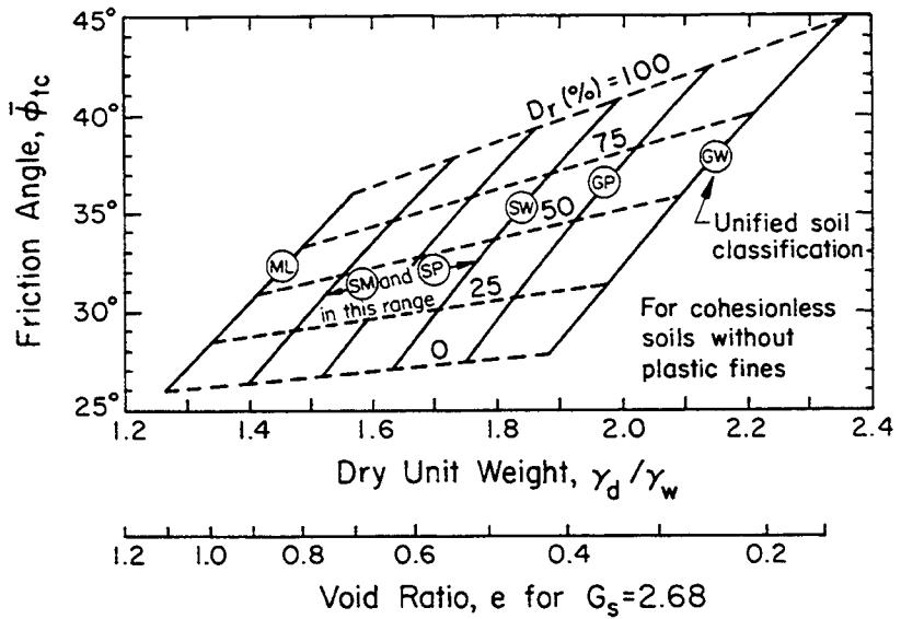
Figure 4-8.  $\bar{\phi}_{tc}$  versus Relative Density and Unit Weight
