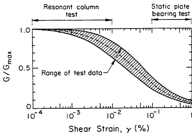
Figure 5-11. Shear Modulus versus Shear Strain for Sands
