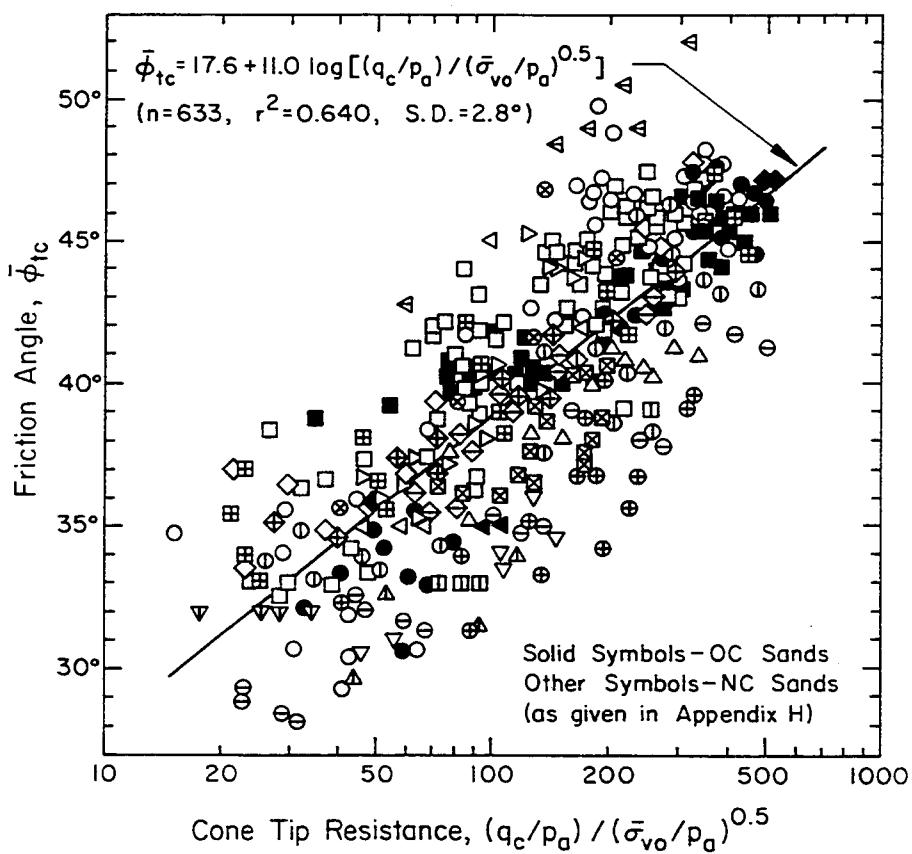
Figure 4-17. Trend of  $\bar{\phi}_{tc}$  with Normalized  $q_c$
