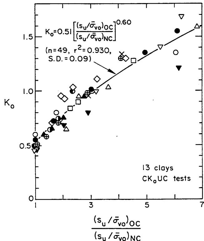
Figure 3-26.  $K_o$  Correlated with Undrained Strength Ratio
