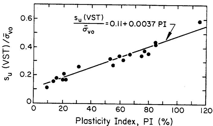
Figure 4-26.  $s_u(VST)/\bar{\sigma}_{vo}$  versus PI for NC Clays
