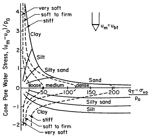
Figure 2-10. Soil Classification Based on CPTU Data
