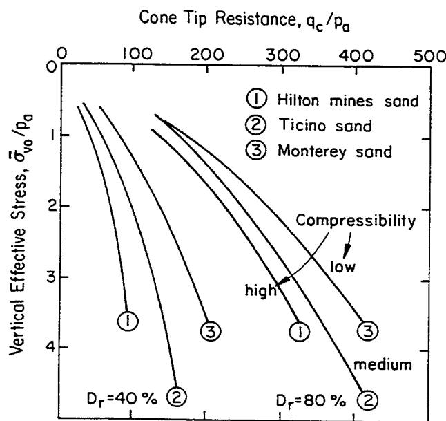
Figure 2-23. Relative Density from CPT, Including Soil Compressibility
