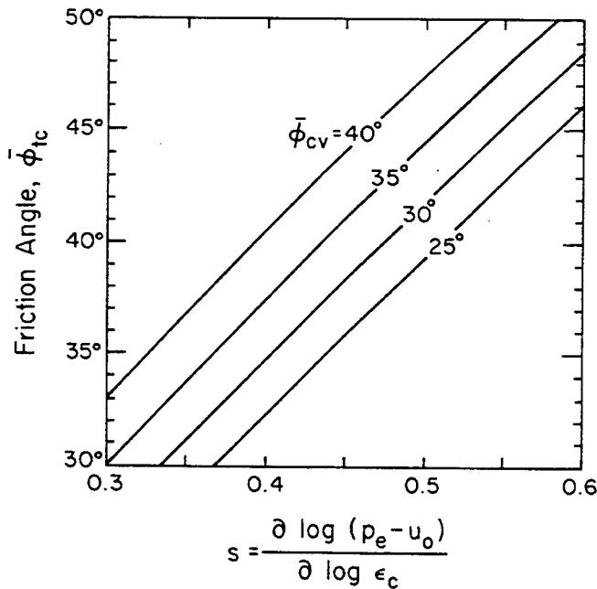
Figure 4-19. Friction Angle Evaluation from PMT Results
