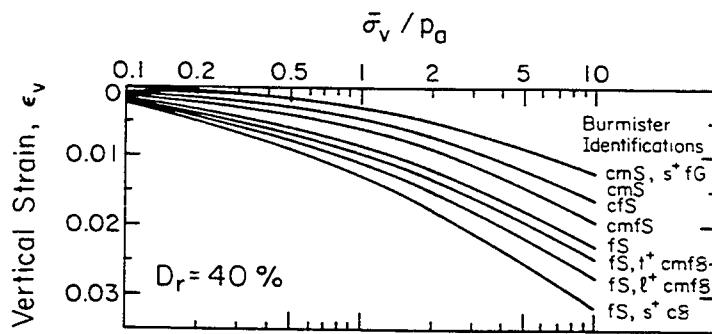
Figure 6-12. Effect of Grain Size on Sand Compressibility
