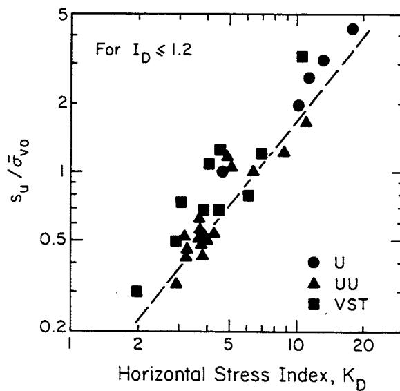
Figure 4-57.  $s_u$  as a Function of  $K_D$  from the DMT
