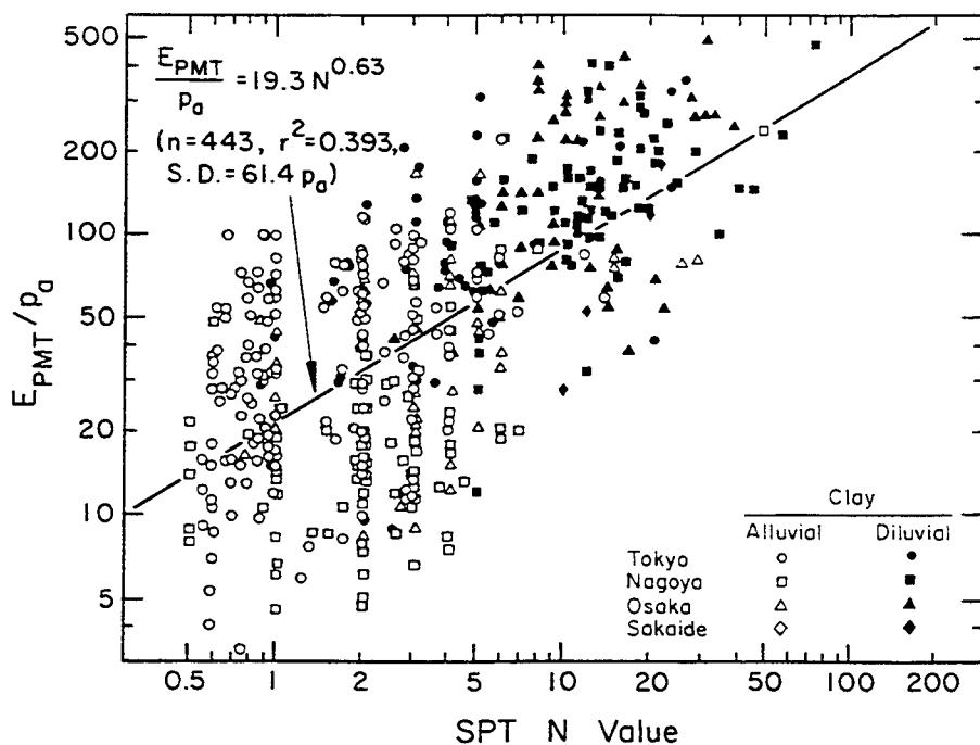
Figure 5-8. PMT Modulus of Clay versus N Value
