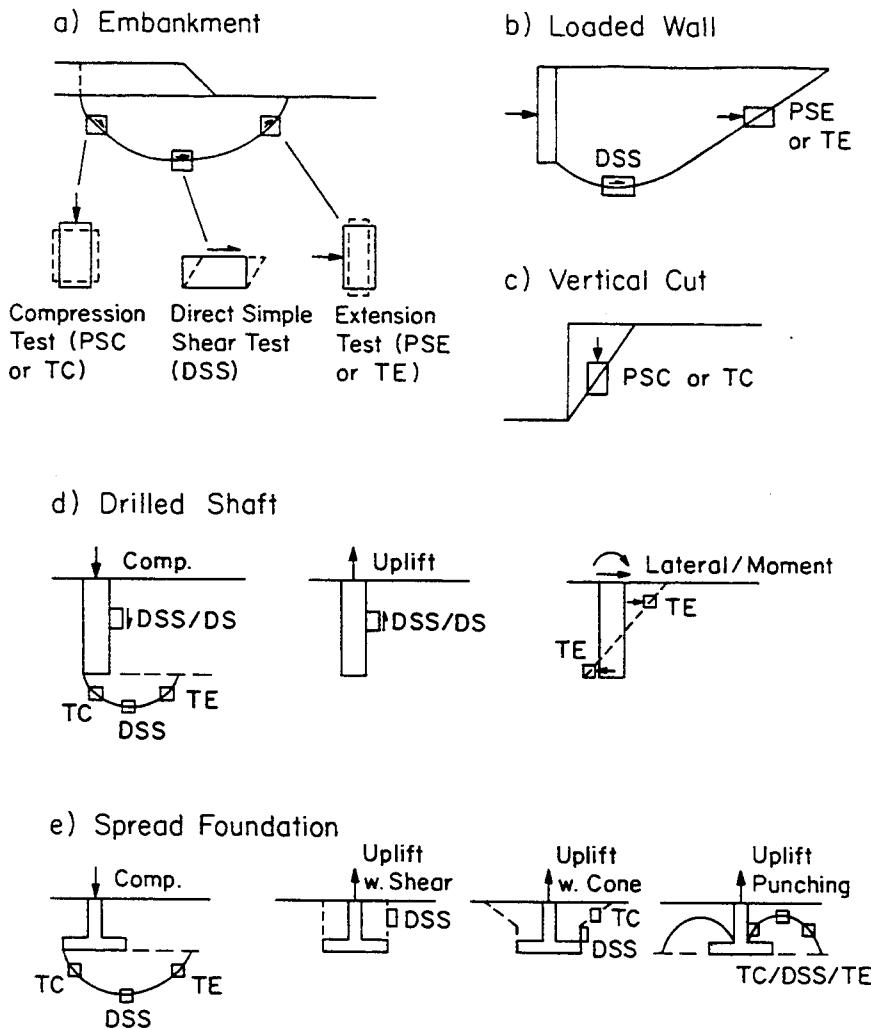
Note: Plane strain tests (PSC/PSE) used for long features
