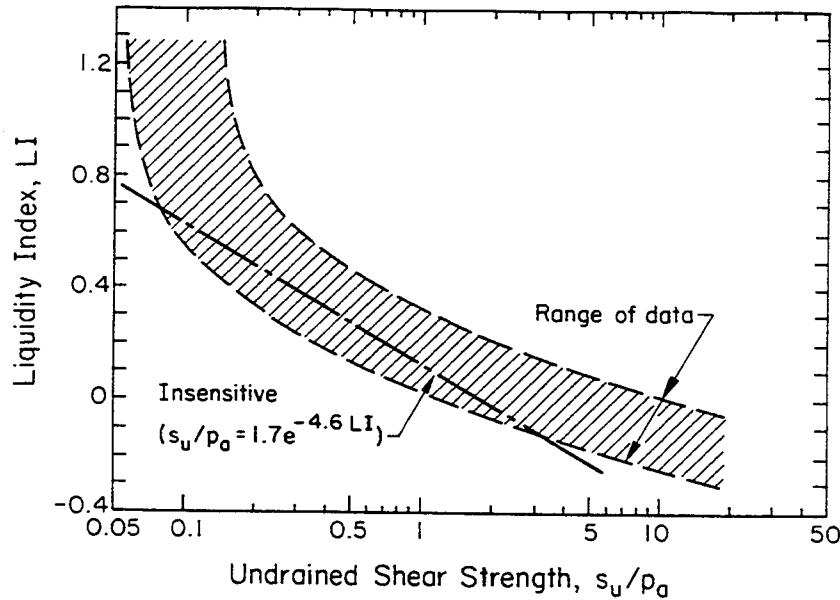
Figure 4-30. Undisturbed Undrained Shear Strength versus LI
