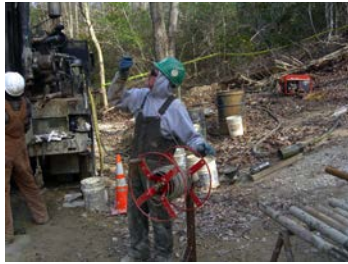
Figure 8: Reel to keep DMT cable from tangling
