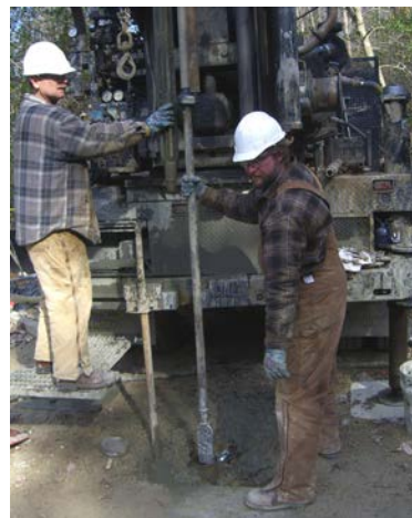
Figure 2: Lowering Torpedo DMT Blade into Borehole
