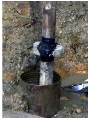
Figure 5: Taping DMT Cable to Outside of Rods Between Steel Centralizer Strips
